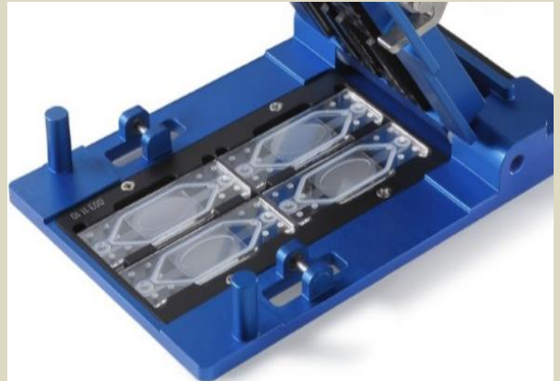
Nasal Airway On Chip for pre-clinical efficacy testing
